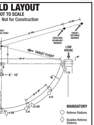
markers plus or minus six inches; target emergence elevation, high house, plus or minus three inches from level of Station 1, low house plus or minus three inchese from level of Station 7. Station levels within plus or minus nine inches of Station 8 level. Mandatory referee positions should be marked.
